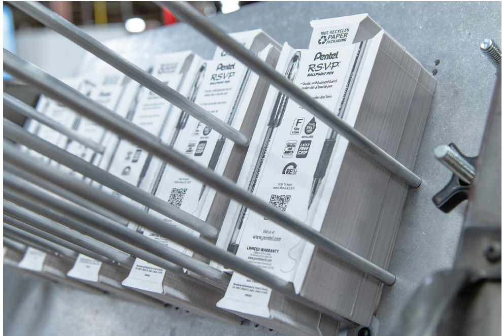
A flat paperboard blank is picked from a magazine and formed into a blister on the equipment.
