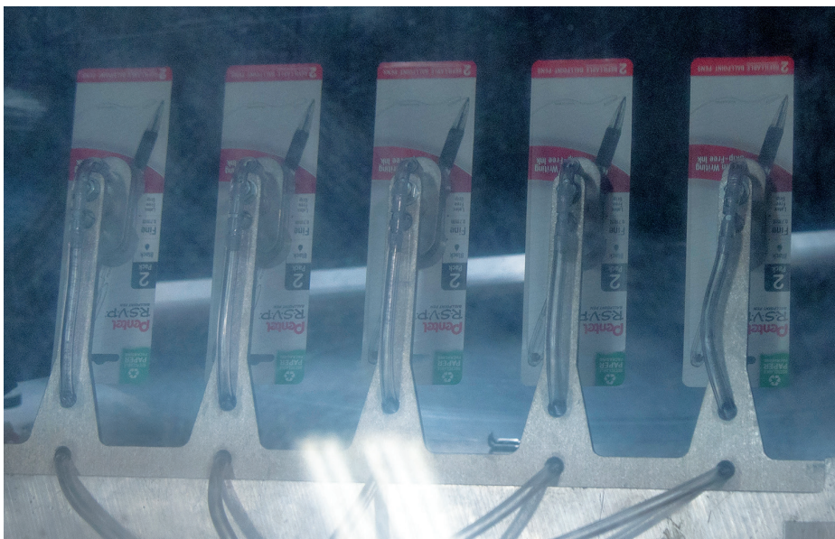
Hanging tab cardstock backing is being applied to the filled paper blister on the retrofitted blister packing equipment here. The backing is intended to be the consumer-facing display portion of the pack when hanging in retail.
